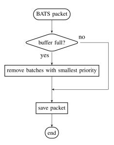
Fig. 8: Flow chart of the receiving procedure in the BF of BATSpro-2 at an intermediate node.
