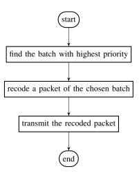
Fig. 9: Flow chart of the transmitting procedure in the BF of BATSpro-2 at an intermediate node.
