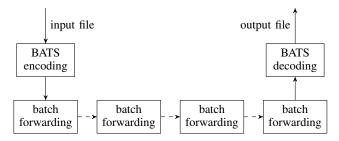
Fig. 3: Structure of a BATS code protocol in the line network in Fig. 1. Each batch forwarding module runs on a network node. The first node includes an encoding module and the last node includes a decoding module.
