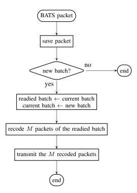
Fig. 5: Flow chart of the batch forwarding module of BATSpro-1 in an intermediate node.
