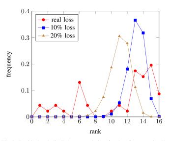
Fig. 7: Empirical rank distribution example in a four-hop line network with real-world packet loss. The two curves marked by 10% and 20% loss are the expected rank distributions of the four-hop line network with 10% and 20% percent independent loss rates, respectively. The average ranks of the three cases are 11.07, 13.13 and 11.12, respectively.
