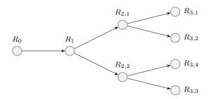
Fig. 2: A tree-type wireless network with multicast links. Node  $R_0$  is the source node, nodes  $R_{3,1}$ ,  $R_{3,2}$ ,  $R_{3,3}$  and  $R_{3,4}$  are the destination nodes, and nodes  $R_1$ ,  $R_{2,1}$  and  $R_{2,2}$  are the intermediate nodes that do not demand the input packets. The two outgoing links of  $R_1/R_{2,1}/R_{2,2}$  share the same wireless channel.
