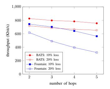
Fig. 6: Compare BATSpro-1 and fountain code protocol when the link loss rate is 10 and 20 percent. For both protocols: K = 5120,  $q = 2^8 T = 1024$ , and the source node transmission rate is 1000 Kbit/s. For BATSpro-1, M = 16.
