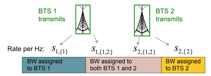
Total rates:  $r_1 = s_{1,\{1\}} x_{\{1\}} + s_{1,\{1,2\}} x_{\{1,2\}}$  $r_2 = s_{2,\{2\}} x_{\{2\}} + s_{2,\{1,2\}} x_{\{1,2\}}$
